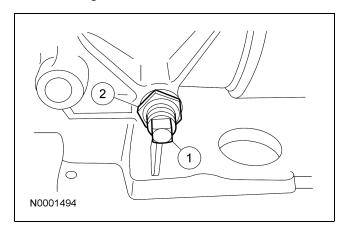
**CAUTION:** Install, but do not tighten, a new locknut on the band adjustment screw. Apply petroleum jelly to the locknut seal.
